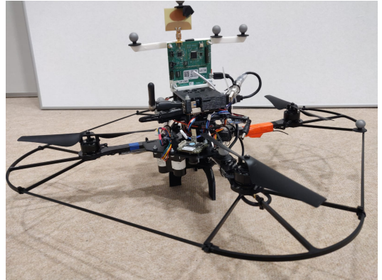
Fig. 1: UAV used for real world experiments with computation board and UWB node.
