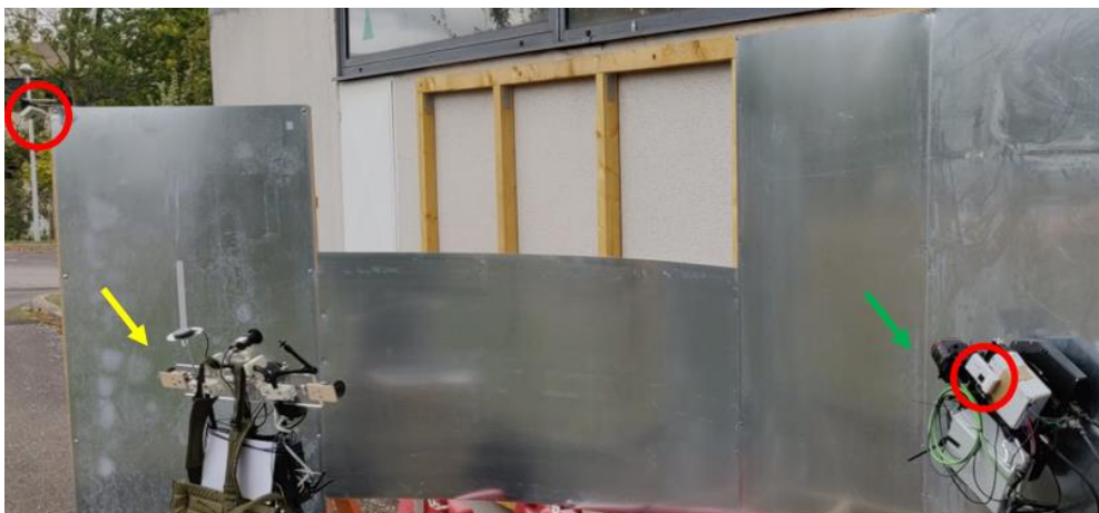
Figure 193: Magnetic crawler robot (green arrow) on a curved metal surface with ultra-wideband localisation (red circles) and laser (yellow arrow) to track the robot for ground truth.
