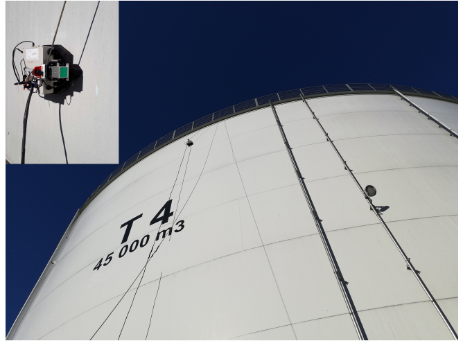
Fig. 1. Crawler Robot Magnetically Attached to a Storage Tank in Bazancourt, France.
