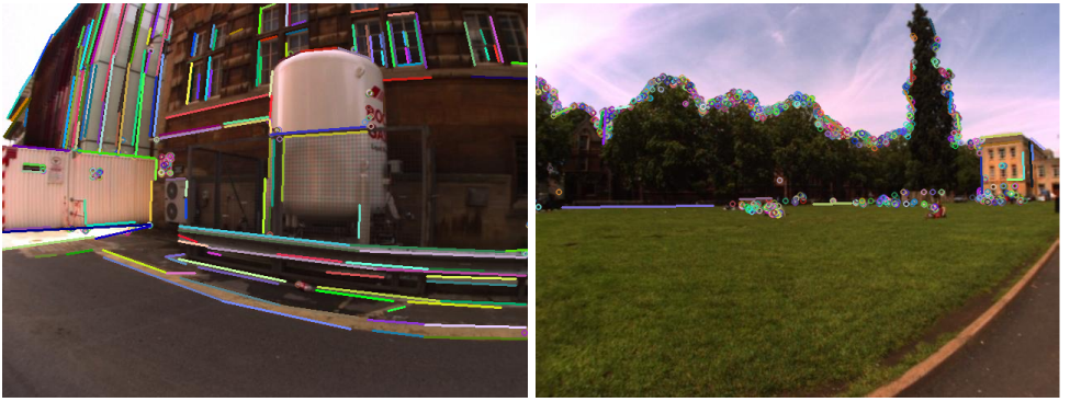
Figure 2: (left) A human-made environment including a high number of lines and a low number of points. (right) An outdoor environment presenting the opposite situation.
