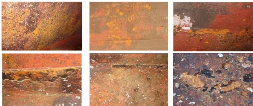
Figure 8: Photographic sequence of hull corrosion
