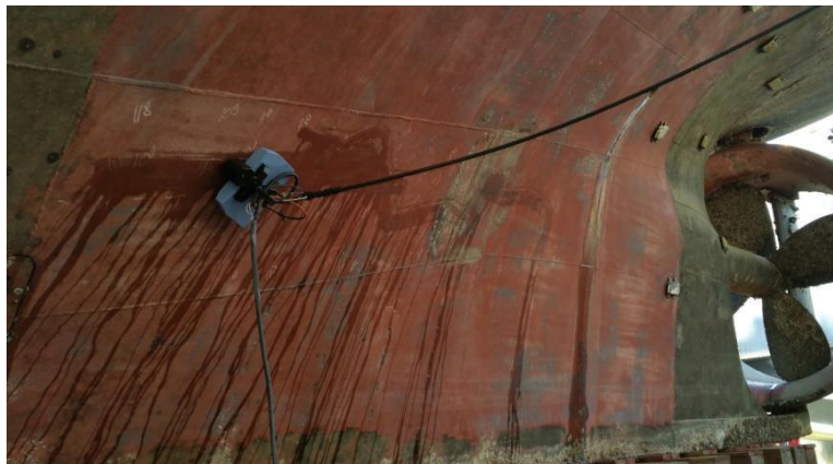
Figure 3: Crawler for hull thickness measurements (Credits: ROBOPLANET)
