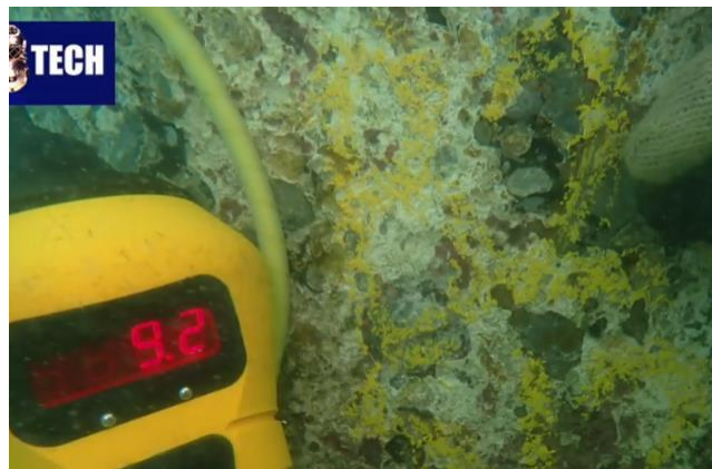
Figure 6: Underwater thickness measurement (Credit: MasterTech Diving Services)
