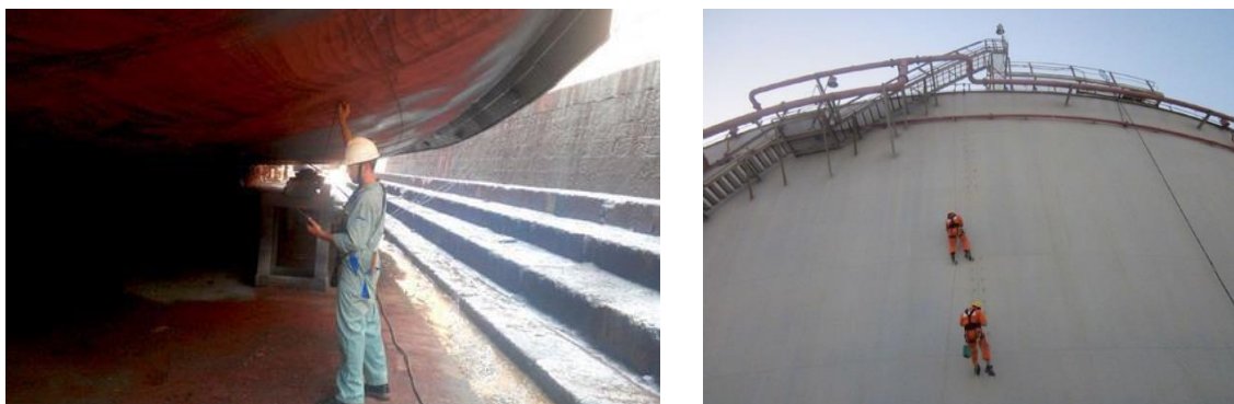
Figure 2: Ship outer hull and storage tank thickness measurements (Credits: P.L Tzaneas & Partners, ROBOPLANET)
