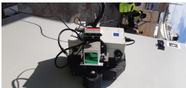
(a) CNRS magnetic crawler
