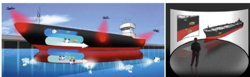
FIGURE 1 Drones, magnetic wheeled crawlers and submersibles working autonomously to visually and acoustically scan a ship while transmitting data to a human operator SOURCE: C PRADALIER, 'AUTONOMOUS ROBOTIC INSPECTION AND MAINTENANCE ON SHIP HULLS AND STORAGE TANKS' (BUGWRIGHT2), DESCRIPTION OF THE ACTION, EU HORIZON 2020 GRANT AGREEMENT NO. 871260, USED WITH PERMISSION
