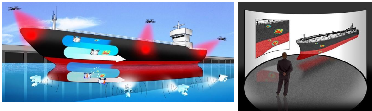
Figure 18: Drones, magnetic wheeled crawlers and submersibles working autonomously to visually and acoustically scan a ship while transmitting data a human operator 10
