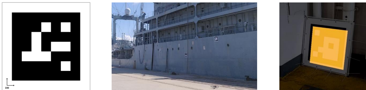
Figure 1: Example ArUco marker (left) and some of the markers mounted on a ship during an integration week in Lisbon '23 (middle). The image on the right shows a tracked overlay over the real marker shown in the HoloLens (note: the offset occurs due to the screenshot process and is not visible in the device itself).
