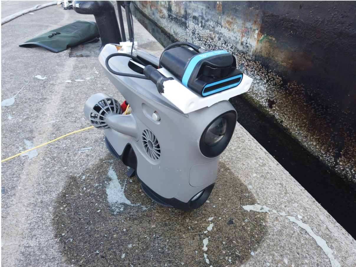
Figure 21: Vehicle involved in hull modelling underwater
