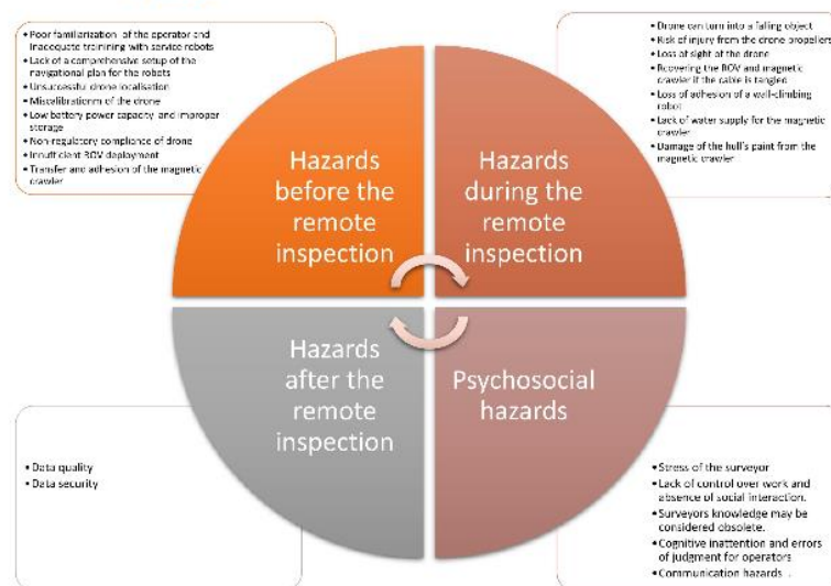
Figure 2. Main hazards during a multi-robot remote inspection.
