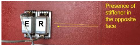
d/ Pseudo pulse-echo configuration for reflection investigation
