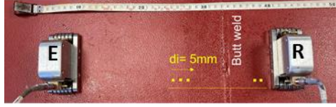
b/ Transmission measurement with the presence of a butt weld
