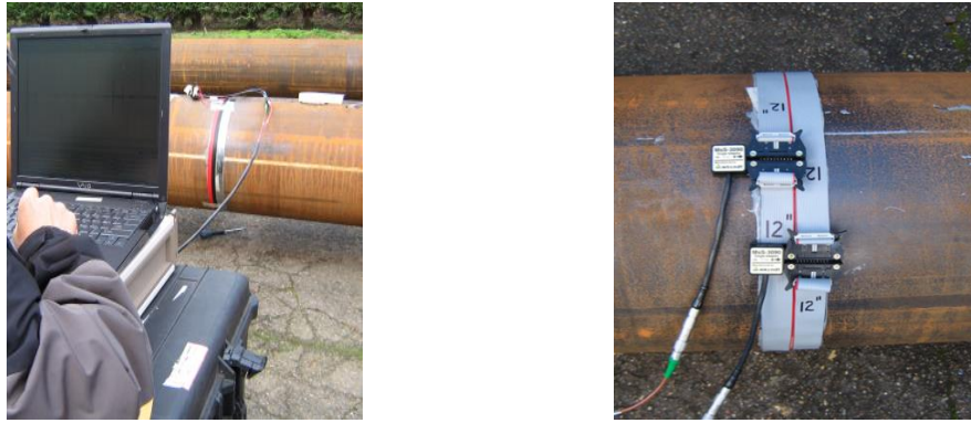
Figure 4: magnetostrictive guided wave system - MsSR3030 (SWRI)
