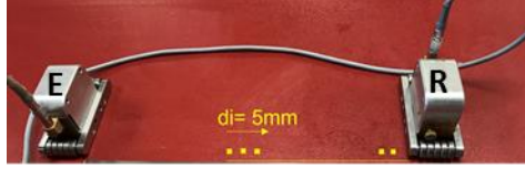
a/ Transmission configuration in a non-defective area ( d_i : probe displacement increment)
